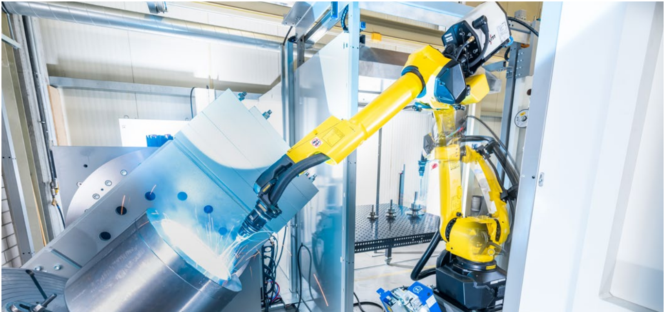
Surfacing of a valve body. The drive 4X wire feeder securely feeds the filler metal on the robot arm.
