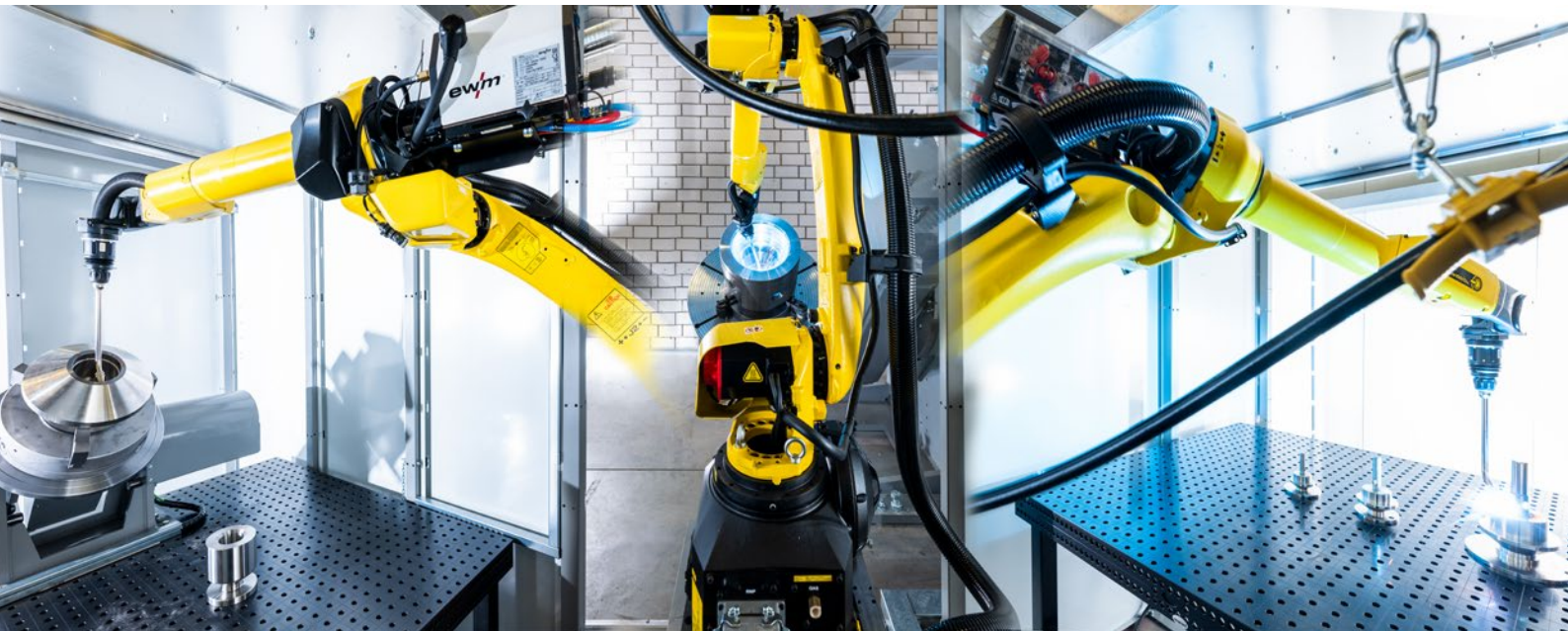
Arrangement of the three work areas of the robot: the large L-positioner with tilting function for the large valve bodies on the left, one small turning/tilting positioner on a system bench for the small valve bodies in the middle, and a third station with a system bench without positioners for any other components.
