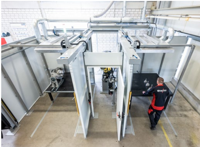
Confined spaces in the design of the robot system with three processing stations
